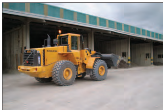
Face shovel loading clay from individual clay storage bins.
